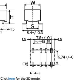
General InformationSeriesUD2StyleSMDDescriptionMiniature Signal Relay, Single<br/>Coil LatchFeaturesSuper-Compact Size, Flat-<br/>PackageRoHSYesCoil TypeSingle Coil (Latching)
