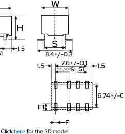
General InformationSeriesUD2StyleSMDDescriptionMiniature Signal Relay, Non-latch<br/>Low Power ConsumptionFeaturesSuper-Compact Size, Flat-<br/>PackageRoHSYesCoil TypeSingle Coil (Non-Latching)
