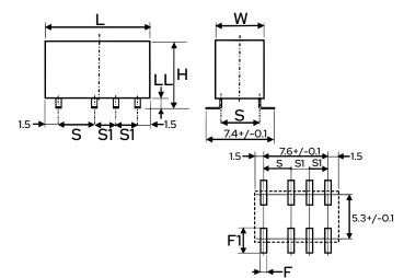
General InformationSeriesUB2StyleSMDDescriptionMiniature Signal Relay, Non-latch<br/>Low Power ConsumptionFeaturesSuper-Compact Size, Flat-<br/>PackageRoHSYesCoil TypeSingle Coil (Non-Latching)
