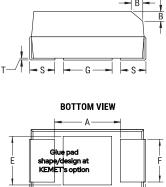
MnO2 Tantalum Dielectric Style SMD Chip Description SMD, MnO2, Molded, Low ESR Features Low ESR RoHS No Prop 65 WARNING: Cancer and reproductive harm https://www.p65warnings.ca.gov SCIP Number 1dd2e1b8-26dd-4d52-927c-6f9 d519011aa Termination Tin Lead (SnPb) AEC-Q200 No **Typical Component Weight** 446.84 mg Shelf Life 156 Weeks MSL 1
