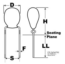
T352 Series Dielectric MnO2 Tantalum Style Radial Description Radial, Solid Tantalum, Conformal, Dipped Low Leakage Features RoHS Yes Termination Tin AEC-Q200 No Construction Conformal Notes Longest Lead Is Positive.
