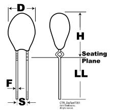
**General Information** T351 Series Dielectric MnO2 Tantalum Style Radial Description Radial, Solid Tantalum, Conformal, Dipped Low Leakage Features RoHS Yes Termination Tin AEC-Q200 No Construction Conformal Notes Longest Lead Is Positive.
