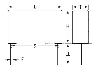
R76 Series Dielectric **Double Metallized** Polypropylene Style Radial Features Pulse RoHS Yes Cut (Tinned Wire) Termination Lead Cut AEC-Q200 No **Typical Component Weight** 13.4 g
