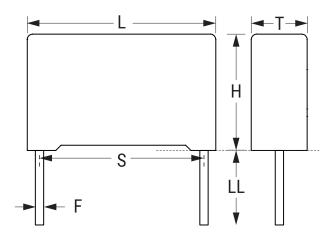
R76 Series Dielectric **Double Metallized** Polypropylene Style Radial Features Pulse RoHS Yes Cut (Tinned Wire) Termination Lead Cut AEC-Q200 No 8.45 g **Typical Component Weight**
