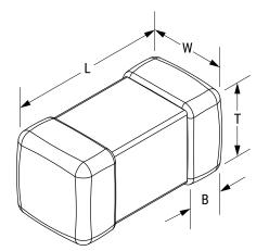
**General Information** Series L-SMS SMD Multi-Layer Style Core Ceramic Description Shielded, Surface Mount Inductor Features Standard Type RoHS Yes Winding Type Multilayer Suggested Replacement -https://www.chilisin.com/en-global/Inductor/Product/BSCL\_ 201209/BSCL00201209R18K Notes 00.
