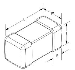
**General Information** L-PMS Series SMD Multi-Layer Style Core Ceramic Description Shielded, Surface Mount Inductor Features Standard Type RoHS Yes Winding Type Multilayer Notes Not recommended for new designs, please see L0805C2R2MPWIT, L0805R2R2MPWRT, L0805C2R2MPWST for replacement.
