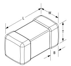
SMD Multi-Layer Style Core Ceramic Description Shielded, Surface Mount Inductor Features Standard Type RoHS Yes Winding Type Multilayer Suggested Replacement -https://www.chilisin.com/en-global/Inductor/Product/BSCL\_ 160808/BSCL00160808R56K Notes 00.
