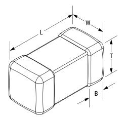
**General Information** Series L-SMS SMD Multi-Layer Style Core Ceramic Description Shielded, Surface Mount Inductor Features Standard Type RoHS Yes Winding Type Multilayer Notes Suggested Replacement https://www.chilisin.com/englobal/Inductor/Product/BSCL\_ 160808/BSCL001608086R8M 00.
