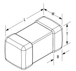
**General Information** Series L-SMS SMD Multi-Layer Style Core Ceramic Description Shielded, Surface Mount Inductor Features Standard Type RoHS Yes Winding Type Multilayer Notes Suggested Replacement https://www.chilisin.com/englobal/Inductor/Product/BSCL\_ 160808/BSCL001608081R5M 00.
