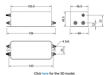
**General Information** FLLE2-U Series Style **Chassis Mount** Description Single Phase, Chassis Mount Filters Single Phase Features Phase Single-phase RoHS Yes Qualifications IEC/EN 60939, UL, CSA AEC-Q200 No Lead Threaded Studs M4 **Terminal Type** Threaded Studs M4 1300 VDC Test Voltage DC (P to N)
