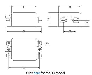
**General Information** FLLE2-P Series Style **Chassis Mount** Description Single Phase, Chassis Mount Filters Features Single Phase Phase Single-phase RoHS Yes Qualifications IEC/EN 60939, UL, CSA AEC-Q200 No Lead Fast On **Terminal Type** Faston Test Voltage DC (P to N) 1300 VDC
