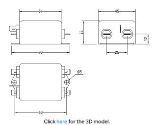
FLLE2-R Series Style **Chassis Mount** Description Single Phase, Chassis Mount Filters Features Single Phase Phase Single-phase RoHS Yes Qualifications IEC/EN 60939, UL, CSA AEC-Q200 No Lead Fast On **Terminal Type** Faston Test Voltage DC (P to N) 1300 VDC
