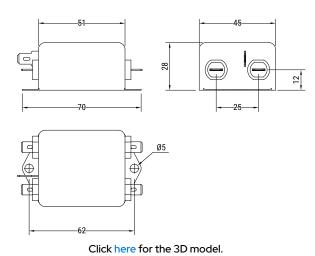
**General Information** FLLE2-R Series Style **Chassis Mount** Description Single Phase, Chassis Mount Filters Features Single Phase Phase Single-phase RoHS Yes Qualifications IEC/EN 60939, UL, CSA AEC-Q200 No Lead Fast On **Terminal Type** Faston Test Voltage DC (P to N) 1300 VDC
