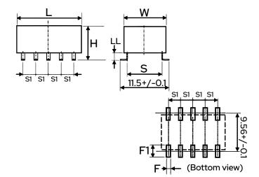
General InformationSeriesEB2StyleSMDDescriptionMiniature Signal Relay, Non-latchFeaturesCompact Size, Flat-Package.<br/>FCC (1500 V) surge capacity. UL<br/>recognized and CSA certified.<br/>Low power consumption<br/>(100-200 mW)RoHSYesCoil TypeSingle Coil (Non-Latching)
