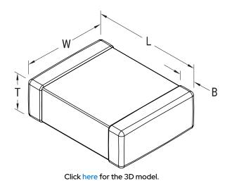
SMD, Fixed, RF, Ultra High Q, Description Low ESR, Class I Ultra High Q, Low ESR, Class I Features RoHS Yes Tin Termination Marking No AEC-Q200 No **Typical Component Weight** 1.37 mg Notes Solder Reflow Only. Shelf Life 78 Weeks MSL 1
