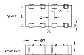
**General Information** Array Comm X7R Flex Series SMD Array Style SMD, MLCC, Array, Flex Termination, Class II Description RoHS Yes Termination Flexible Termination AEC-Q200 No Chip Size 0612 MSL
