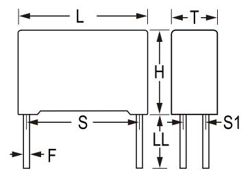
**General Information** C4AU Series Dielectric Metallized Polypropylene Style Radial Features DC Filtering RoHS Yes Lead 4 Wire Leads Qualifications AEC-Q200, IEC61071, EN61071, VDE0560 AEC-Q200 Yes **Typical Component Weight** 93.7 g Rth = 14 C/W. Miscellaneous
