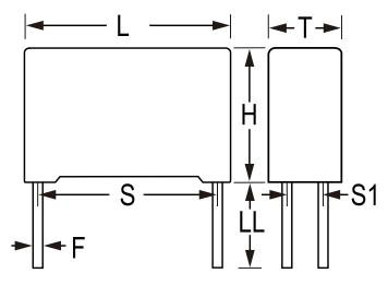
**General Information** C4AU Series Dielectric Metallized Polypropylene Style Radial Features DC Filtering RoHS Yes Lead 4 Wire Leads Qualifications AEC-Q200, IEC61071, EN61071, VDE0560 AEC-Q200 Yes **Typical Component Weight** 64.6 g Rth = 18 C/W. Miscellaneous
