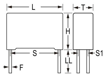
**General Information** C4AU Series Dielectric Metallized Polypropylene Style Radial Features DC Filtering RoHS Yes Lead 4 Wire Leads Qualifications AEC-Q200, IEC61071, EN61071, VDE0560 AEC-Q200 Yes **Typical Component Weight** 80.6 g Rth = 15 C/W. Miscellaneous
