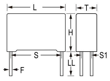
**General Information** C4AU Series Dielectric Metallized Polypropylene Style Radial Features DC Filtering RoHS Yes Lead 4 Wire Leads Qualifications AEC-Q200, IEC61071, EN61071, VDE0560 AEC-Q200 Yes **Typical Component Weight** 93.2 g Rth = 14 C/W. Miscellaneous
