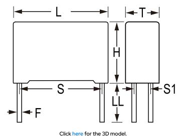
**General Information** C4AQ-P Series Dielectric Metallized Polypropylene Style Radial Features DC Filtering RoHS Yes Lead 4 Wire Leads Qualifications AEC-Q200, IEC61071, EN61071, VDE0560 AEC-Q200 Yes **Typical Component Weight** 134.1 g Rth = 10 C/W. Miscellaneous
