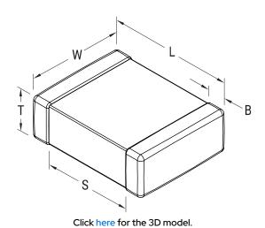
**General Information** Series SMD Comm X5R Style SMD Chip SMD, MLCC, Temperature Stable, Class II Description Features Temperature Stable, Class II RoHS Yes Termination Tin Marking No AEC-Q200 No **Typical Component Weight** 1.21 mg Shelf Life 78 Weeks MSL 1
