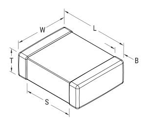
SMD Comm U2J Series SMD Chip Style Description SMD, MLCC, Ultra-Stable, Low Loss, Class I Features Ultra-Stable, Low Loss, Class I RoHS Yes Termination Tin Marking No AEC-Q200 No **Typical Component Weight** 1.06 mg Shelf Life 78 Weeks MSL 1
