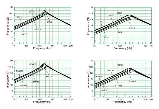
AC Line Filters - Common Mode SS Coils, 20H Series
