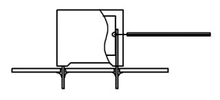
Temperature monitored inside the capacitor.
