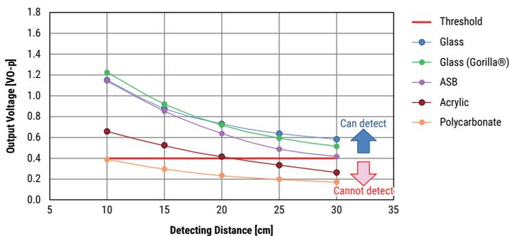
Measuring conditions: Transfer velocity - 1 m/s
