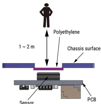
Detecting distance increased to a few meters by using a polyethylene plate.
