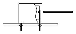
Temperature monitored inside the capacitor.
