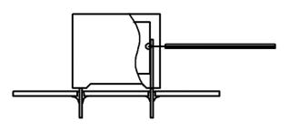
Temperature monitored inside the capacitor.
