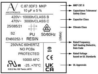
(data): Manufacturing Plant, Date Code, Day of Production, Internal Mark UL810: Applicable if inline with "Marking" from page 1
