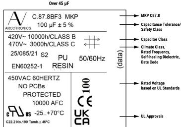
(data): Manufacturing Plant, Date Code, Day of Production, Internal Mark UL810: Applicable if inline with "Marking" from page 1
