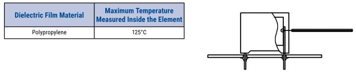
Temperature monitored inside the capacitor.
