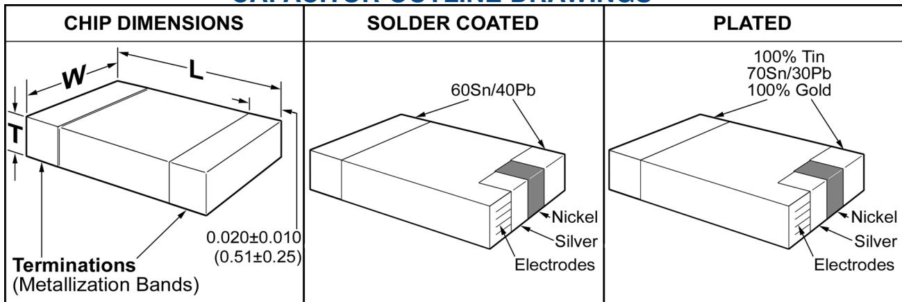
\*Add .38mm (.015") to the positive width and thickness tolerance dimensions and .64mm (.025") to the positive length tolerance dimension for the Sn60 solder coated product.
