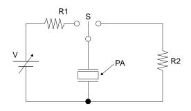
Protective resistor R1=1k $\Omega$ Protective resistor R2=1k $\Omega$ Polarizing conditions: DC voltage application  $0V\rightarrow150\pm0.2V$  (to be retained for 10 seconds)  $\rightarrow0$
