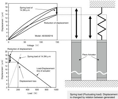
is changed by relation between generated force and spring constant of actuator.
