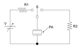
$\begin{array}{l} Protective\ resistor\ R1=1k\Omega\\ Protective\ resistor\ R2=1k\Omega\\ Polarizing\ conditions:\ DC\ voltage\ application\\ 0V{\rightarrow}150{\pm}0.2V\ (to\ be\ retained\ for\ 10\ seconds){\rightarrow}0 \end{array}$
