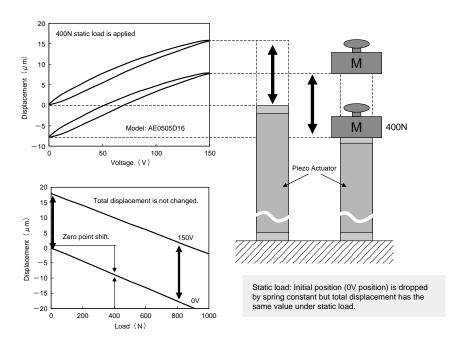
Fluctuating load: Load value changes by spring reaction when actuator moves.
